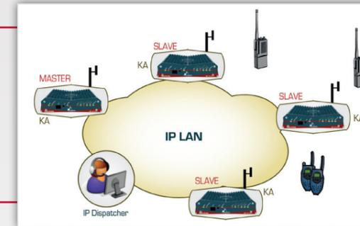
**Base station IP-linked.** The KA-XXX supports IP connections among the base stations to realize multisite hierarchical systems. The role of a device can be set as Master, Secondary Master, Slave or Backup Master. A Master manages up to 32 Slaves/Secondary Master.
