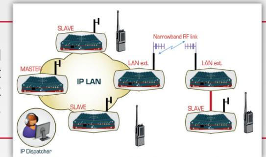
**Single site TIER 3 trunking system.** Adding the TIER3 Controller to a group of KA-XXX, the channels can be efficiently shared between all users according to the ETSI standard TIER3 Trunking protocol.
