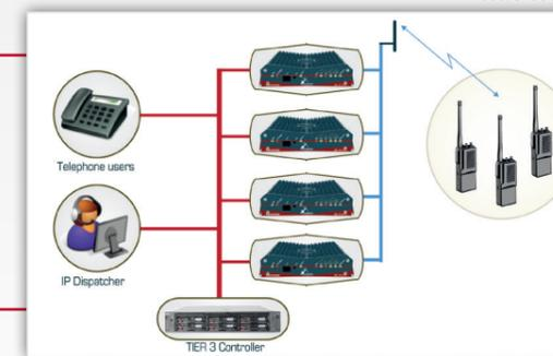
**Multisite simulcast TIER 3 trunking system.** The TIER3 Controller can manage a group of IP-linked simulcast networks realizing a wide-area trunking system.
